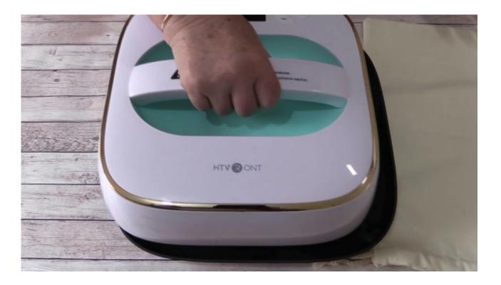
For projects that require heavy pressure, there are hand holds on the sides of the machine. These hand holds allow you to easily apply more pressure as required, and you can pick the machine up using the hand holds to place the machine onto your project and back onto the stand when you have finished pressing the vinyl. These side handles are ideal if you have problems picking things up one handed.
